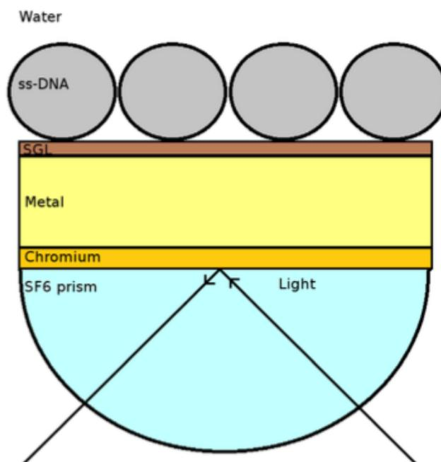
**Figure 1.** Schematic model of SPR biosensors based on a single graphene layer (SGL) and noble metals. A noble metal is deposited on a SF6 prism substrate with a chromium layer of 2 nm interposed. The SGL (0.34 nm) is on the top of the metal and acts as a biomolecular recognition element (BRE) as well as a protective layer.
