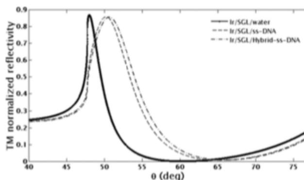
**Figure 2.** ISPR coupling features for  $S_{Ir}$  in water (black line) and during the DNA detection (dashed lines).
