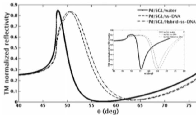
**Figure 3.** ISPR signal of the  $S_{Pd}$  biosensors in water (black line) and during the (ds)-DNA formation (dashed lines). We note that the peak shift is still appreciable for the two states of DNA.
