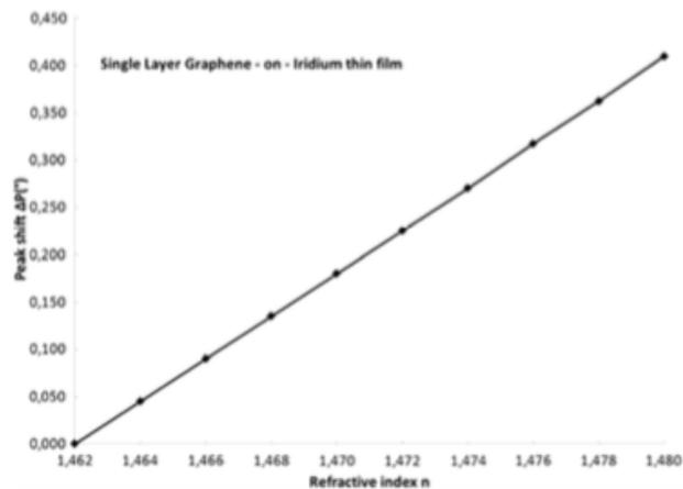
**Figure 4.** Sensitivity of the  $S_{Ir}$  SPR sensor during the ss-DNA hybridization.
